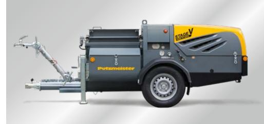
Compliant with Stage V emission standard, the SP 11 THF can easily cover distances of 80 m or heights of 40 m. The sieve and vibrator have been improved to achieve a continuous material flow, even when conveying screed containing plastic or metal fibres. The maximum delivery rate of 15 m<sup>3</sup>/h and the installed equipment provide all you need to professionally convey self levelling floor screed.
